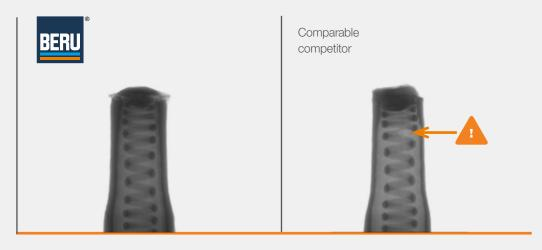
The thread spiral doesn't break, and passes the life cycle test with ease
